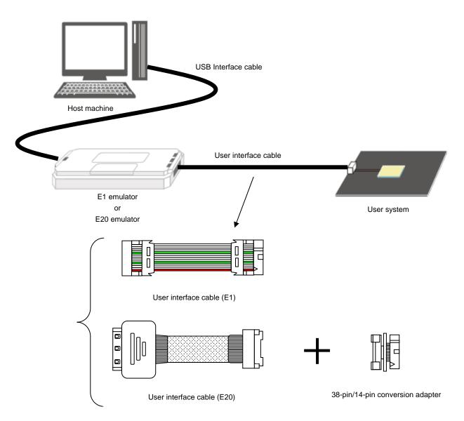
**Remark** To use it with the E20, connect the 38-pin/14-pin conversion adapter to the user interface cable (E20). 38-pin is not supported.
