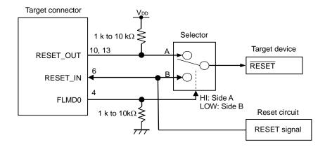
**Remark** FLMD0 is high level when E1/E20 is connected, and FLMD0 is pulled down when MINICUBE2 is not connected.
