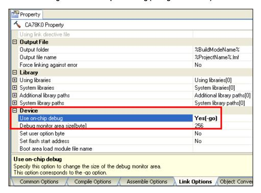
Figure 2-19. Link Option Setting (Debug Monitor Area)
