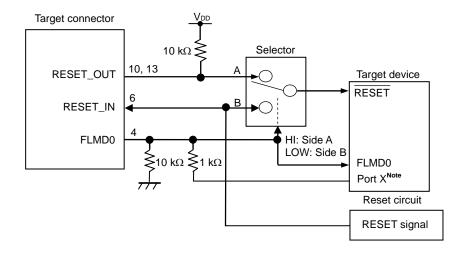
Note This circuit is designed for flash self programming, which controls the FLMD0 pin via ports.
