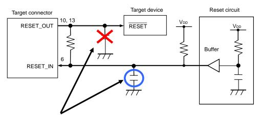
If a capacitance element such as a capacitor or resistor is connected to the RESET\_OUT pin, the target device might not be able to communicate with E1. If necessary, connect a capacitor to the RESET\_IN pin.
