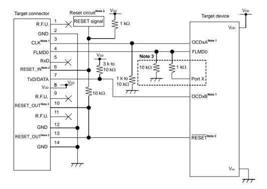
Figure 2-6. Only Debugging Is Performed (OCDxA, OCDxB Communication x = 0, 1)
