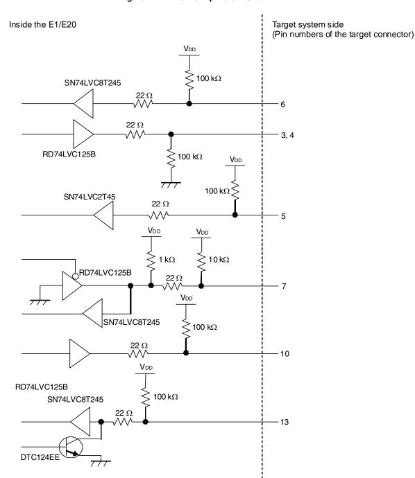
Figure A-1. E1/E20 Equivalent Circuit
