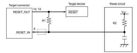
Figure 2-10. Circuit Connection with Reset Circuit That Contains No Buffers
