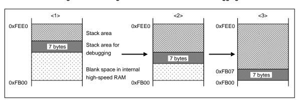
Figure 2-22. Change in Address of Stack Area for Debugging
